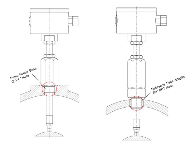
1. For the installation of the Probe Holder Base of the Probe Mount KS016, a thread hole G 3/4" in the bearing housing, exactly positioned to the measuring point, and a machined mounting surface are required.
